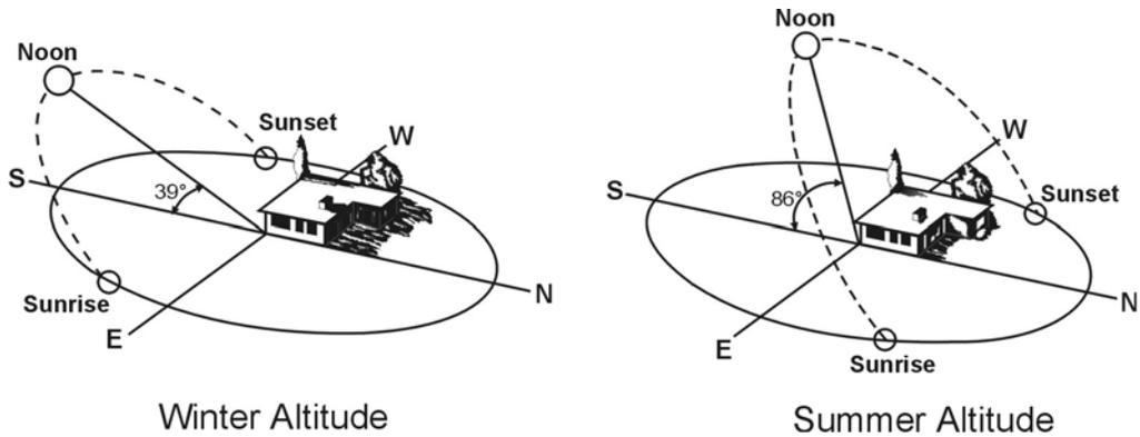
Figure 5. Sun Path Diagrams for 28° N. Latitude
